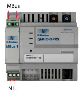
For correct function, the MBus 1 module and gMUC must be installed immediately next to each other.
